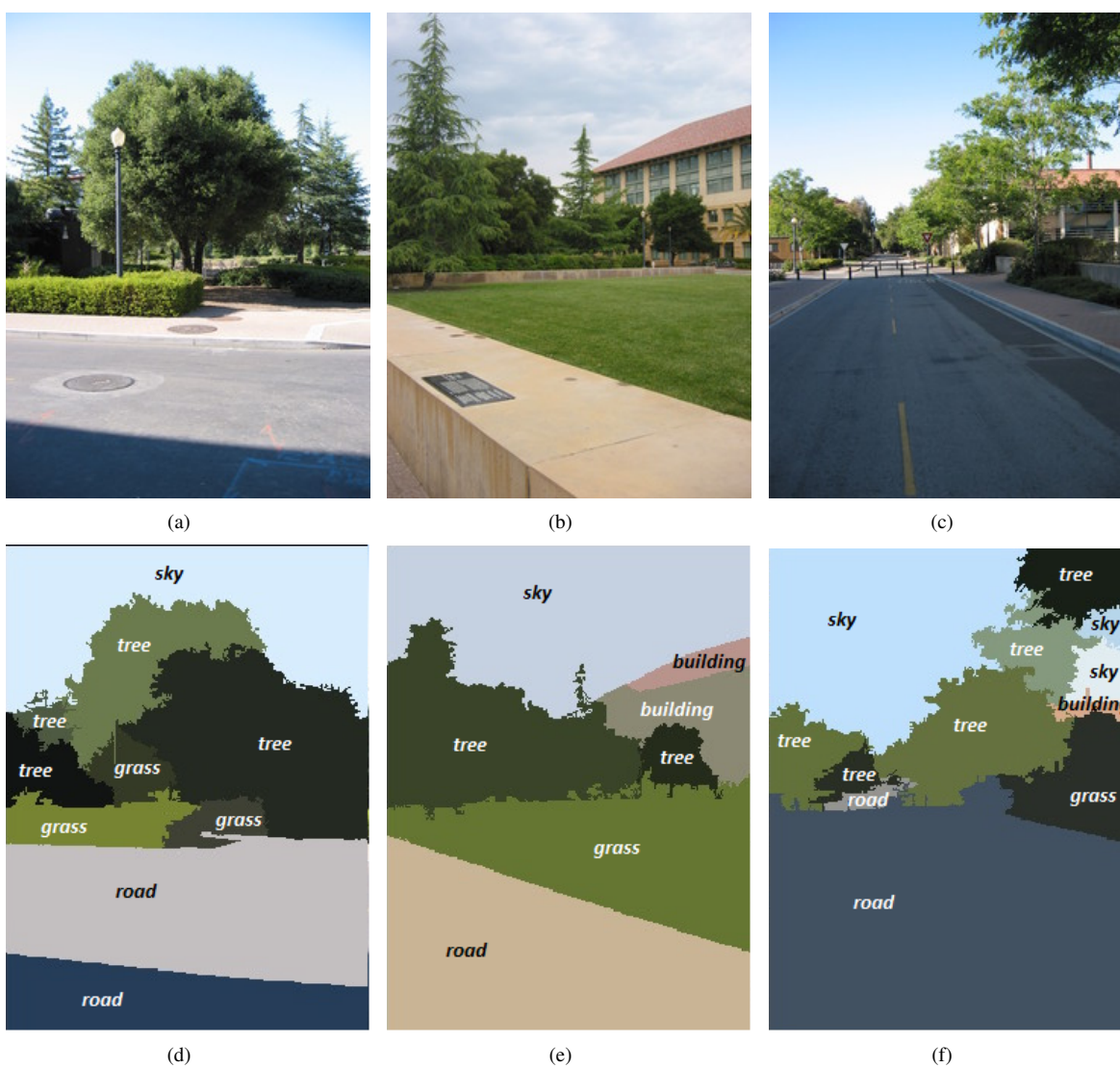
Figure 2: Semantic segmentation on test images using the bag of words representation extended by color statistics, and the Naïve Bayesian classifier.
