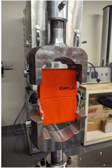
Fig. 1 Setup of the elongation testing of the substrate fabric with the MTS Alliance RF/200 traction apparatus.
