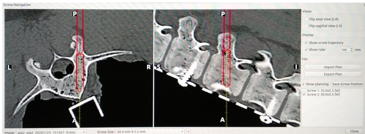
Figure 2. IBIS software: Snapshot from intraoperative use of navigated tap. The tool tip and the expected screw trajectory are shown in solid red lines, and the saved trajectory is shown in dotted lines.
