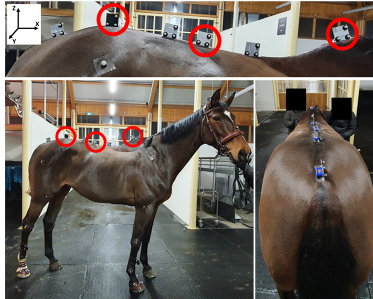
Figure 1. IMU and marker localization on the horse.
