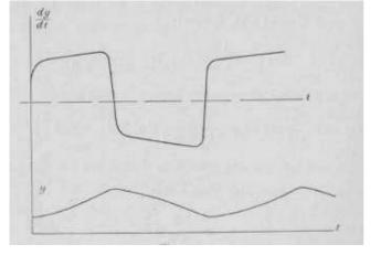
Fig. 1. Solution of Rocard's jerk equation (4).
