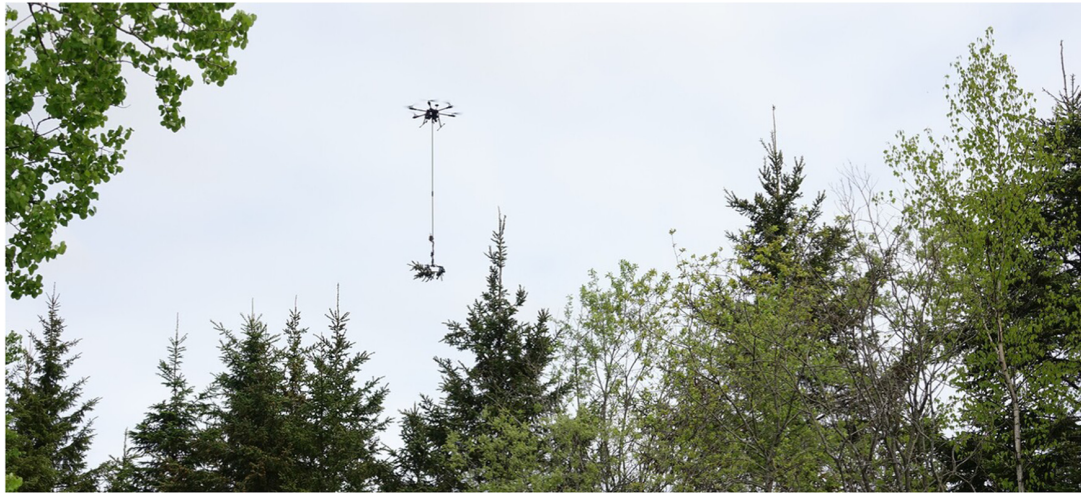
Fig. 1. Unmanned aerial vehicle equipped with the DeLeaves tool after collecting a red spruce ( Picea rubens ) sample in Quebec.
