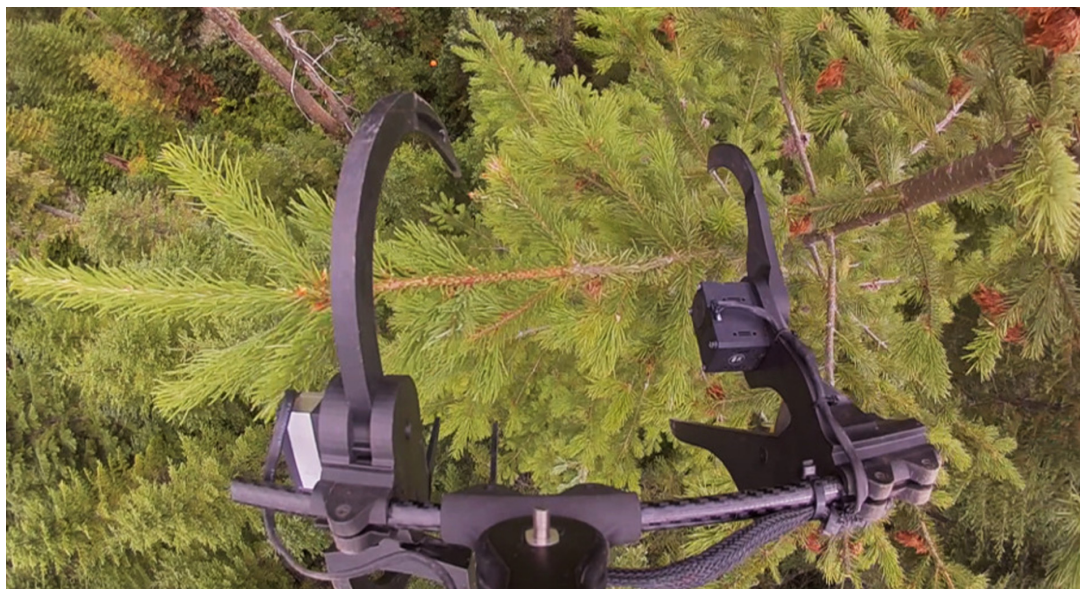
Fig. 12. View from DeLeaves's camera before collecting a branch from a 40-m Douglas Fir.
