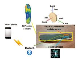
Figure 3: The system architecture of Smart Insole System [18].
