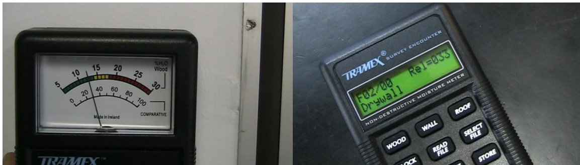
Figure 1 a & b: The analog moisture meter besides its more sophisticated digital counterpart.
